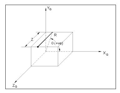
Figure 1.3 : Cylindrical Coordinate System
