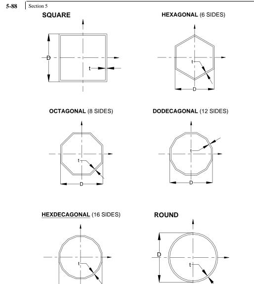
Figure 5.12 - Prismatic Tapered Tube Shapes
