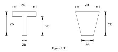
To define a concrete member, the user must not provide AX, but instead, provide YD and ZD for a rectangular section and just YD for a circular section. If no moment of inertia or shear stiffness areas are provided, the program will automatically calculate these from YD and ZD.
