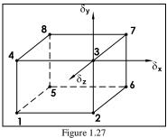
By collapsing various nodes together, an eight noded solid element can be degenerated to the following forms with four to seven nodes. Joints 1, 2, and 3 must be retained as a triangle.
