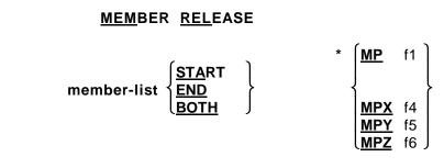
See Section 1.8 where  $f_1$  = release factor for all 3 moments; or enter  $f_4$ ,  $f_5$ , and/or  $f_6$  as release factors for each moment separately. The moment related stiffness co-efficient will be multiplied by a factor of  $(1-f_1)$  at the specified end. Release factors must be in the range of 0.001 through 0.999.
