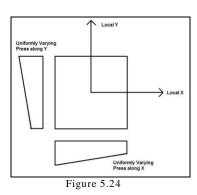
Center of the element is considered as the origin defining the rectangular area on which the pressure is applied.
