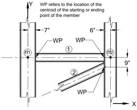
$f_1$ ,  $f_2$ , and  $f_3$  correspond to the distance, measured in LOCALized or Global coordinate system, from the joint (START or END as specified) to the centroid of the starting or ending point of the members listed. MEMBER OFFSET command can be
