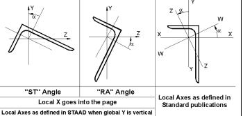
Figure 1.6a - Local axis system for various cross sections when global Y axis is vertical. NOTE: The local x-axis of the above sections is going into the paper
