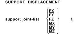
*See Section* 1.16.7 FX, FY, FZ specify translational displacements in X, Y, and Z directions respectively. MX, MY, MZ specify rotational displacements in X, Y, and Z directions.
