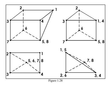
The stiffness matrix of the solid element is evaluated by numerical integration with eight Gauss-Legendre points. To facilitate the numerical integration, the geometry of the element is expressed by interpolating functions using natural coordinate system, (r,s,t) of the element with its origin at the center of gravity. The interpolating functions are shown below:
