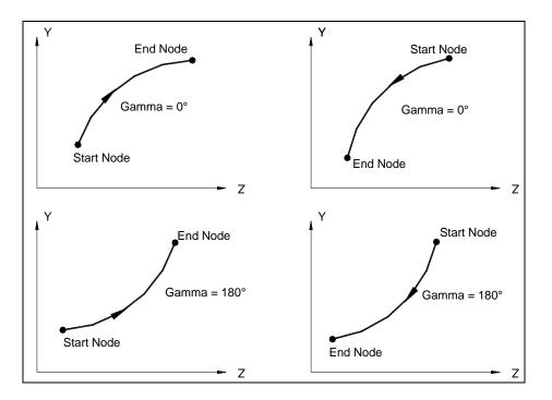
Gamma angle for various configurations of the circular arc lying in the global YZ plane
