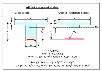
A typical screen from the STAAD beam design output, showing the cracked moment of inertia value, is shown below.
