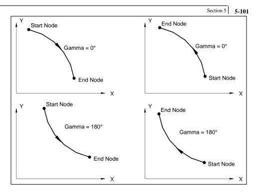
Gamma angle for various configurations of the circular arc lying in the global XY plane
