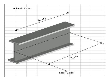
Figure 2.1 - Terms used in calculating slenderness ratios KL/r for local Y and Z axes
