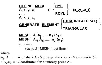
If CYL or RCYL is defined, above coordinates will be in cylindrical or reverse cylindrical coordinates system. Optional coordinates  $x_0$ ,  $y_0$  and  $z_0$  will be the cartesian coordinates for the origin of the cylindrical coordinates. Defaults to 0, 0, 0 if not provided. The 3 fields (x, y, z) may be replaced by a joint number whose coordinates have been defined in the JOINT COORDINATE command by entering
