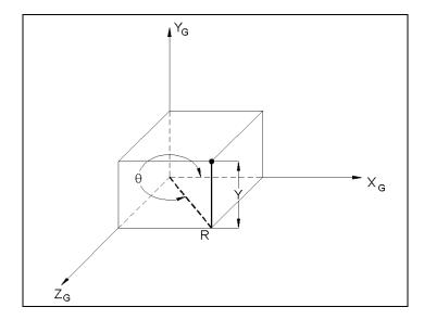
Figure 1.4 : Reverse Cylindrical Coordinate System
