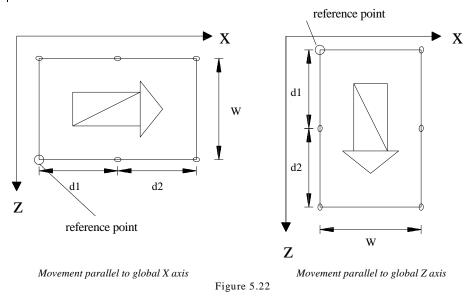
Notice that in the left view, the reference point is on the positive Z wheel track side; whereas in the right view, the reference point is on the least positive X wheel track side.
