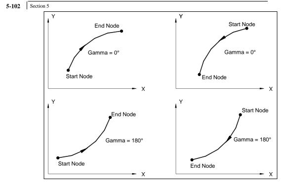
Gamma angle for various configurations of the circular arc lying in the global XY plane
