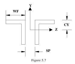
**Note:** The parameter RVV is defined as the radius of gyration about the minor principal axis for single angles - z-z axis for "TA ST" angles, and y-y axis for "TA RA" angles.
