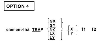
This is for applying a trapezoidally varying load with the following characteristics:
