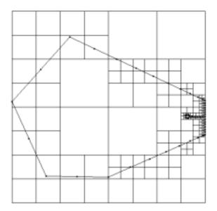
Figure 2: Initial quadtree of model.
