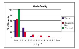
Figure 17: Histogram of element quality for the square model.
