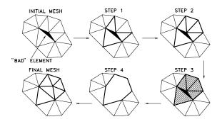
Figure 9: Back-tracking procedure to remesh around a "bad" element.
