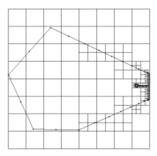
Figure 3: Quadtree of model after forcing largest cell size at boundary.
