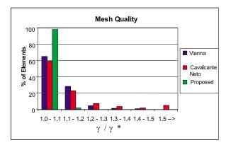
Figure 18: Histogram of element quality for the circle model.
