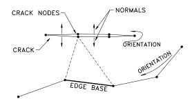
Figure 7: Selection of a candidate node at a crack edge.
