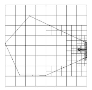
Figure 4: Quadtree of model after forcing maximum of one level of difference.
