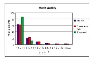
Figure 19: Histogram of element quality for the stand model.
