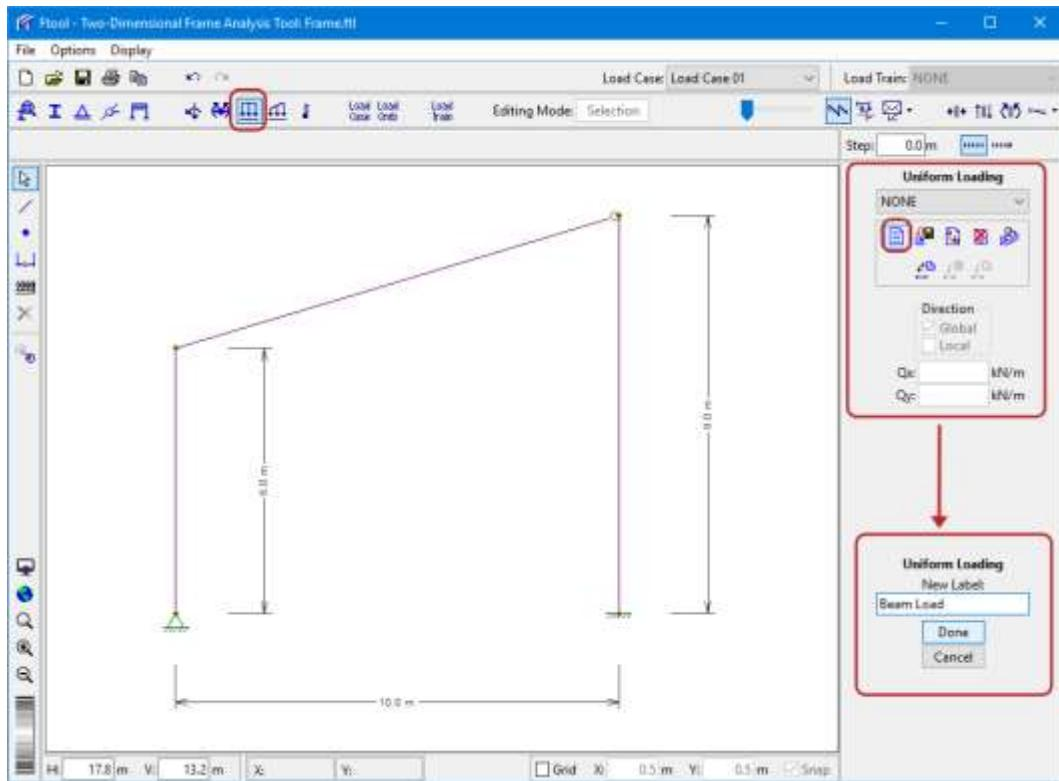
**Definition of value of uniformly distributed force load and assignment to beam member in local system**
