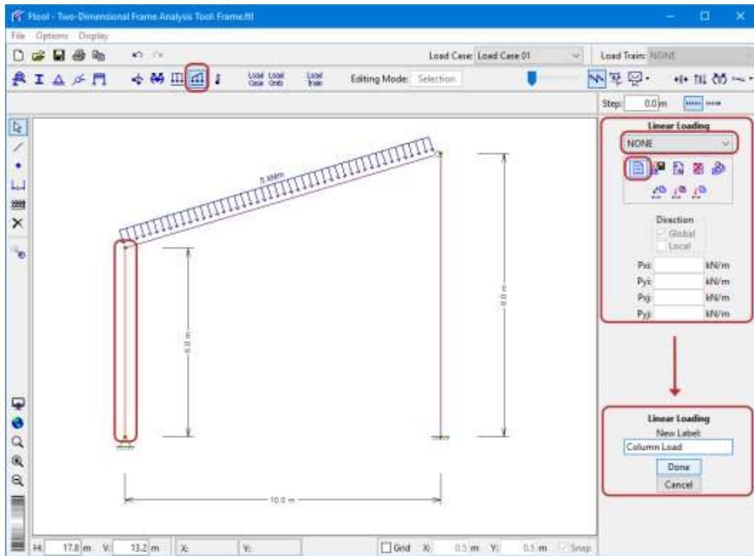
**Definition of values of linearly distributed force load and assignment to right column member in global system**
