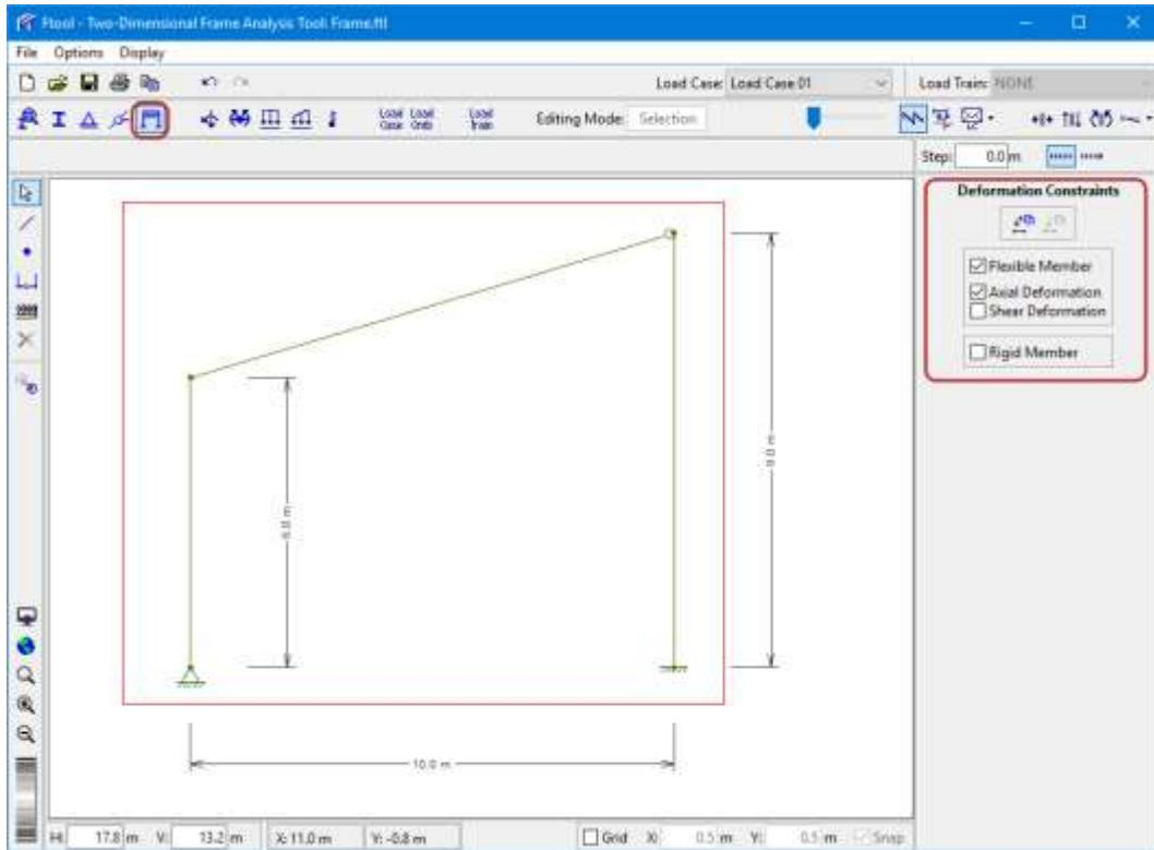
Turn on shear deformation and assignment to selected members
