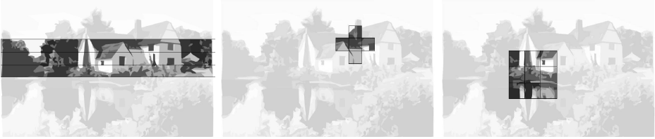
Figure 4.4: Different sliding window configurations. The crisper areas of the pictures represent the image regions actually present in main memory.
