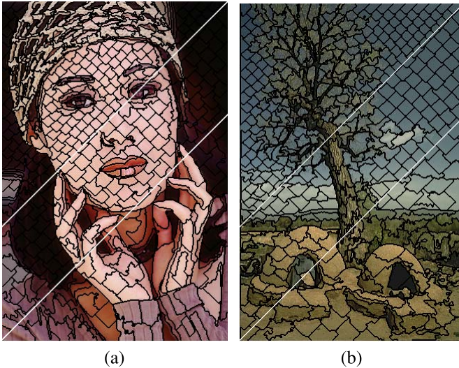
Fig. 1. Results by our real-time DBSCAN superpixel method. Here the numbers of superpixels are about 250, 450, and 900 in the regions separated by two white parallel lines.
