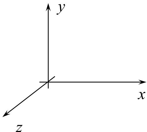
$$\begin{bmatrix} x' \\ y' \\ z' \\ 1 \end{bmatrix} = \left[ \begin{array}{cccc|c} 1 & 0 & 0 & t_x \\ 0 & 1 & 0 & t_y \\ 0 & 0 & 1 & t_z \\ \hline 0 & 0 & 0 & 1 \end{array} \right] \begin{bmatrix} x \\ y \\ z \\ 1 \end{bmatrix}$$
