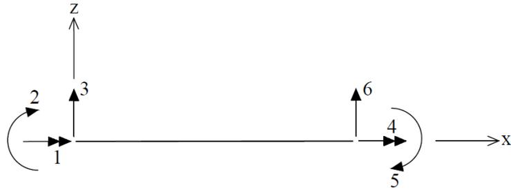
**Figure 2.10** Degrees of freedom numbering order of a grillage element
