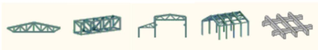
**Figure 2.1** Different types of linear element models (analysis models): plane truss, spatial truss, plane frame, spatial frame and grillage
