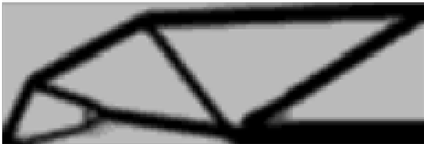
Figure 4.3: MBB-Beam by stress constrained topology optimization
