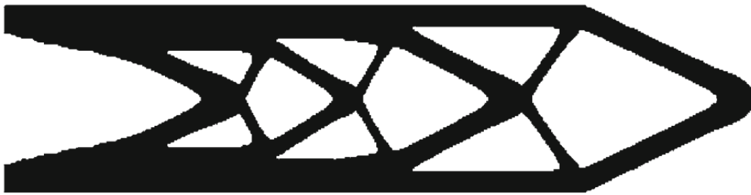
Figure 4.12: Standard topology optimization for the long cantilever beam [66]
