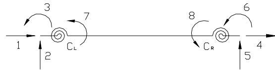
Fig. 2: 2-D Beam element with springs on its extremities. Auxiliary Global system.
