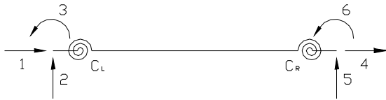
Fig. 1: 2-D Beam element with springs on its extremities. Global system.
