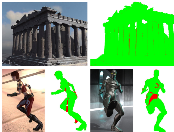
Figure 1: Real-time rendering applications exhibit a considerable amount of spatio-temporal coherence. This is true for camera motions (top) as well as for animated object (bottom). The snapshots of the Parthenon, Heroine, and Ninja sequences illustrate this fact. Newly visible surface points are rendered in red, whereas the vast majority (shown in green) were previously visible. This paper introduces a real-time method that exploits this coherence by caching and tracking visible surface information.
