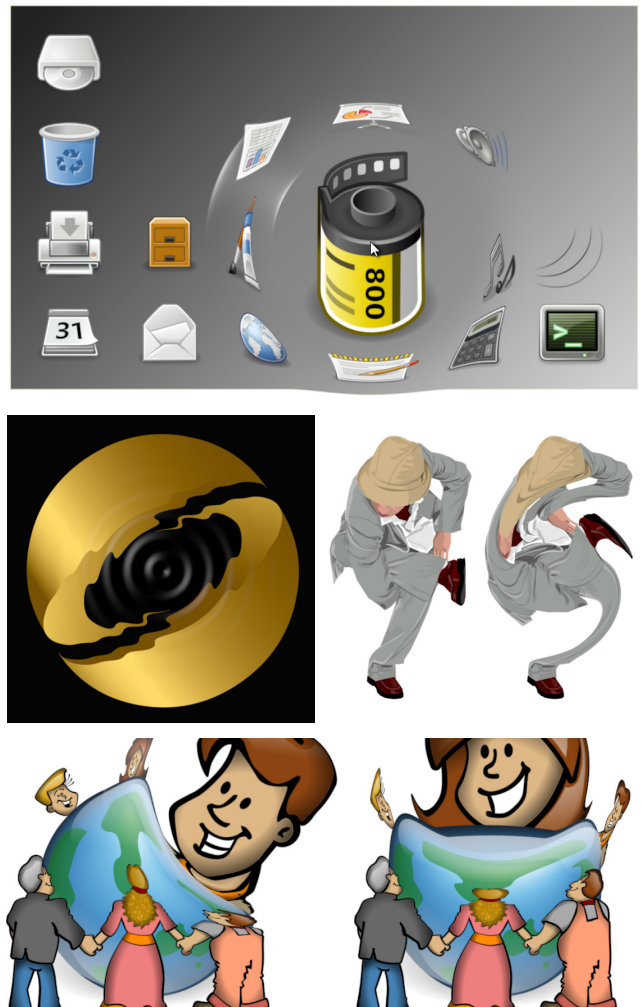
Figure 20: Parametric warps. By perturbing the texture coordinates prior to rendering, we can produce distortion effects that are gaining popularity in modern user interfaces, while retaining the crispness and resolution-independence of the vector graphics description.
