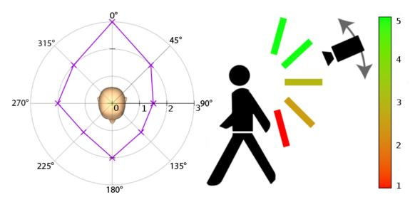
Figure 2.6: User preferences according to Kosch et al. experiment [43] regarding camera position and orientation. The Left side indicates user preferences along the x-axis. Right side indicates orientation preferred on the y-axis
