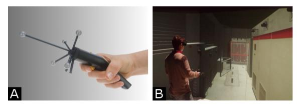
Figure 2.14: Devices used to control virtual techniques : (A) Flystick (B) Tablet with 6DoF Tracking
