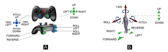
Figure 2.21: Chen et al [20] tests two different techniques for 6DoF direction control: (A) Joystick-Based Controller. (B) Head-Based Controller
