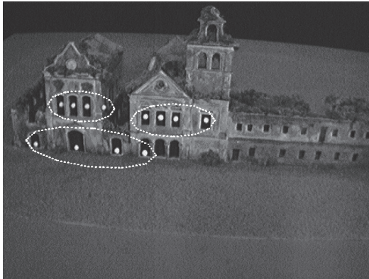
Figure 10: Convent mockup with 3 collinear patterns of markers, to be used for an AR visualization.
