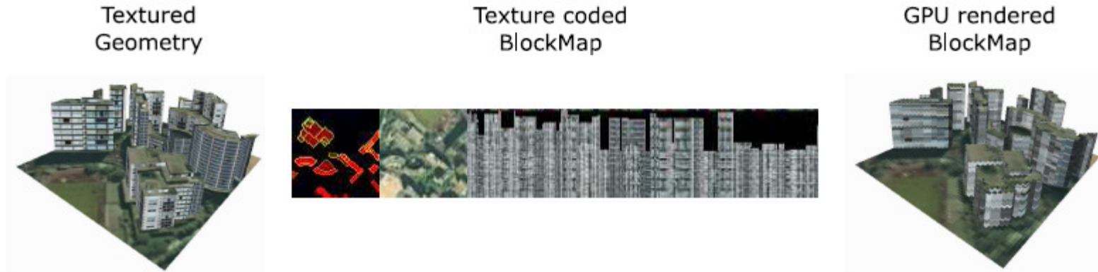
Figure 1: The BlockMaps idea: replace far away groups of buildings with a concise texture-based representation, called BlockMap, which is efficiently rendered by a GPU ray caster.
