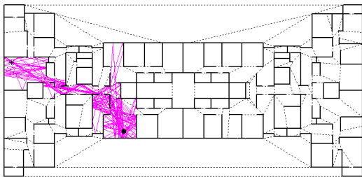
Figure 7: A few propagation paths computed for the residential building example
