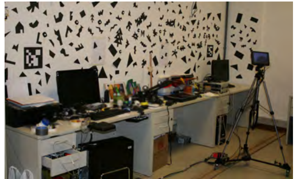
Figure 4: Test station for low precision mode. There are two markers on the wall. The camera and a portable monitor were placed on a tripod which is on top of a dolly (camera cart).
