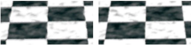
Figure 6: Comparison of signal drift for a simple round-robin subpixel update sequence (left) and our irregular sequence (right).
