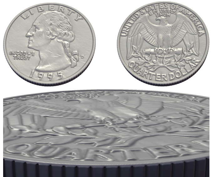
Figure 10: Full model optimization, with geometry and normals from a variety of sources. A model of a quarter was produced from initially flat geometry and a bump map. The figure shows optimized model with normals recomputed from geometry.
