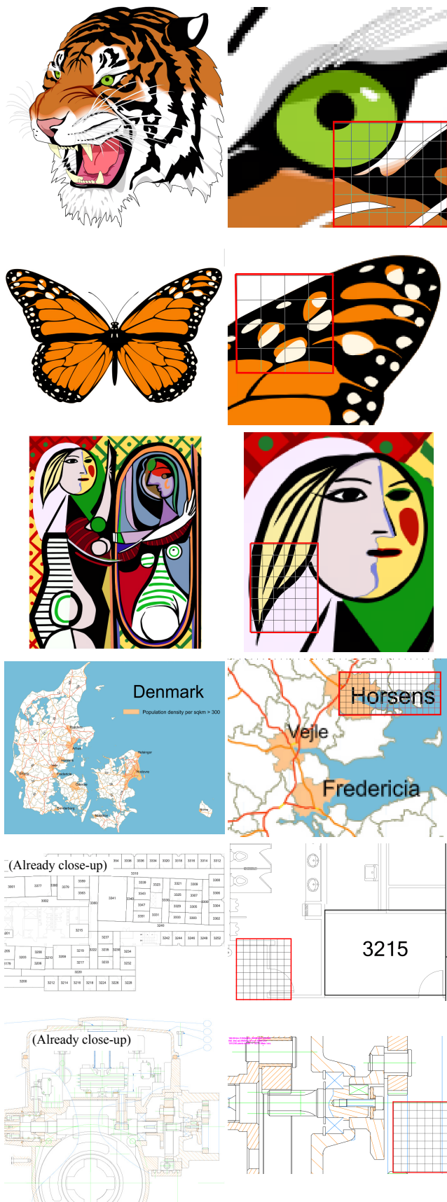
Figure 16: Example results, and close-ups showing good anti-aliasing. Inset images reveal cell grid and magnified graphics.
