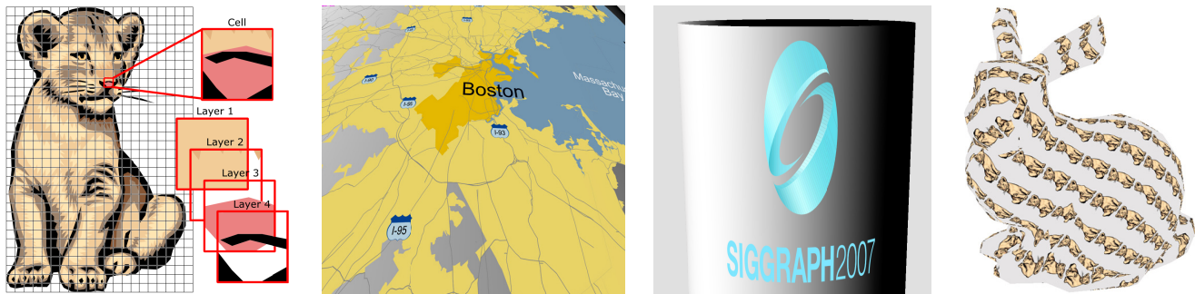
Figure 1: Within each cell of a coarse grid, a texel program encodes several layers of locally specialized graphics primitives, to enable rendering of general vector graphics over arbitrary surfaces, as well as efficient antialiasing.
