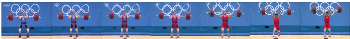
Figure 12: In this video morph result, the shift in the Olympic rings in the background makes it impossible to properly align both the foreground and background elements using the same smooth mapping.
