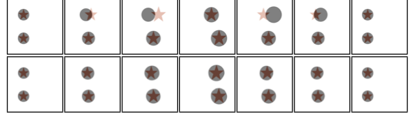
Figure 3: Example showing two input videos simply blended together (top) and blended after temporal synchronization (bottom).
