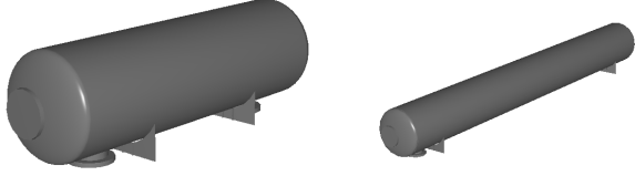
Fig. 6. Output generated by production rule tank . On the left with length = 8 and on the right length = 20. Note that both objects have the same cylinder radius, the size difference is due to different viewing perspectives.
