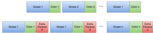
Fig. 5. Layout of the buffer to send to GPU to render parametric surfaces. Above the buffer for normalized primitives and below for primitives that need additional parameters.
