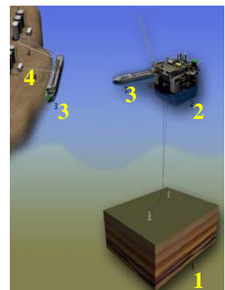
Figure 1: (1) reservoir; (2) offshore platform; (3) transportation ships; (4) oil pipelines.
