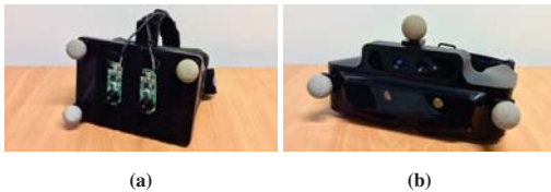
Figure 1: See-Through approaches evaluated: (a) Video See-Through with Oculus Rift; (b) Optical See-Through with Meta Glasses.
