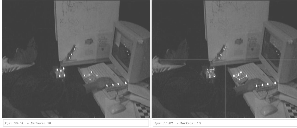
Fig. 2. Optical tracking test with two patterns of each type in the image.
