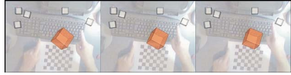
Figure 4. The two-handed OP_TRANSLATE operation is based on two HAND_POSTURE_POINTING postures. An example of CCW rotation is shown.
