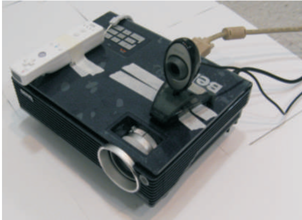
Figure 2 – Projector–camera system used in AR X-Ray.
