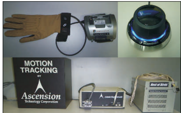
Figure 4. Example of devices supported by the EnCIMA engine: data glove, 3D mouse, and 3D tracker.
