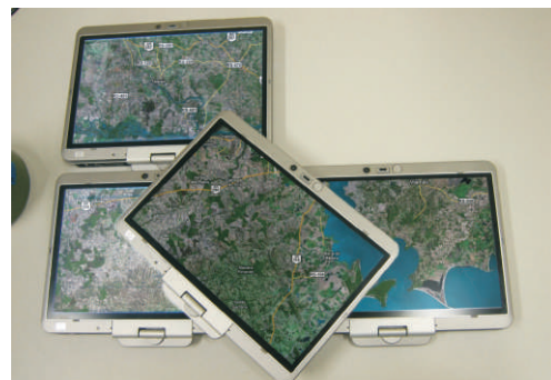
Figure 4. The picture remains continuous even with the displays overlapping.
