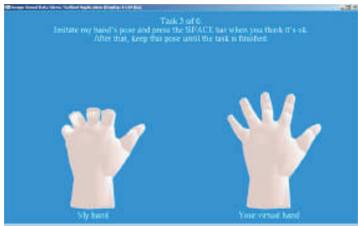
Figure 6. Testbed application showing a task executed by the user. The right hand corresponds to the hand of the user when using the data glove. The left hand means the computer controlled hand holding a pose which must be imitated by the user.
