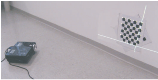
Figure 4. Correspondences between images in projector image coordinates and real world coordinates used in projector calibration.
