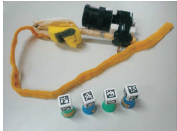
Figure 2. The Image-based Data Glove Prototype. The camera support (a wooden stick) is attached in the hand palm of the user with a Velcro strip (yellow). Thimbles are placed in fingers tips, while the camera is located in the other extremity of the stick, 23 cm far from the fingers tips.
