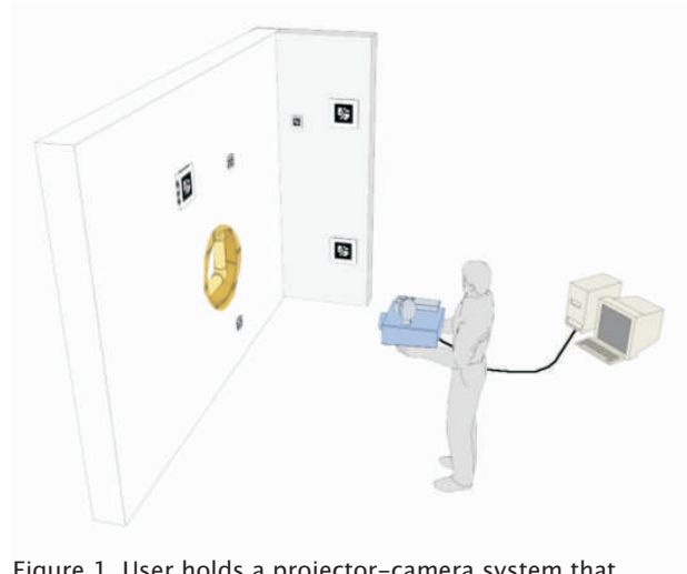
Figure 1. User holds a projector-camera system that delivers the augmentation with proper registration.
