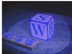
Image seen by a head tracked user standing to the right of a cube located on the surface of the bench display.
