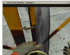
Fig. 10 When the trainee forgets to open one of the levers, the petrol and benzene can overflow.
