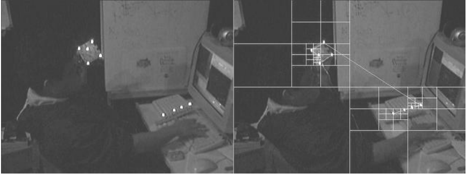
Fig. 1. Grouping for image coordinates of our patterns done with a quadtree
